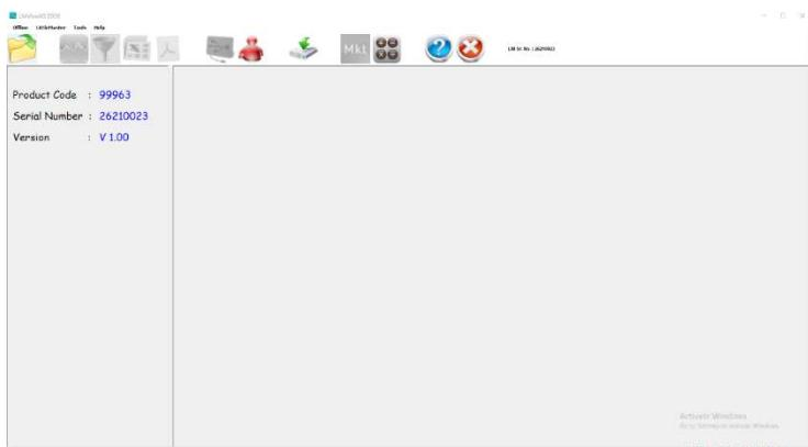
4. After downloading the data, left hand side panel shows Device information- Product code, Serial No. & the firmware Version of the device; right hand side panel shows downloaded data in tabular form.
